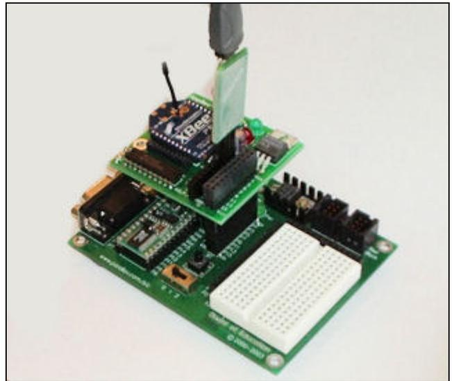
**XBee-PRO mounted on AppBee-MOD
